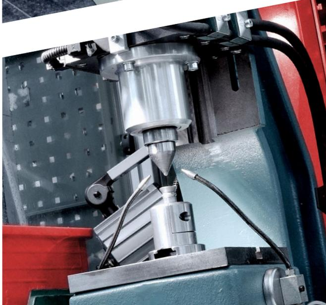
To complete the sequence of inspections, the tube systematically undergoes extremely rigid destructive tests that verify the mechanical strength. Tests are performed in accordance with standard rules and internal procedures of the quality system.
